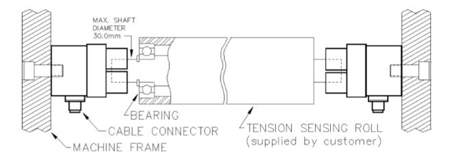
Remove the top half of the transducer shaft clamp by removing the 4 shaft clamp screws.
